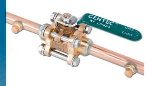
Our dual-port ball valves are full-port, double seal, ball-type three-piece design with forged bronze/brass body and chrome-plated brass ball. Only 1/4 turn of the handle is required to operate the valve from the fully open to the fully closed position. All valves are serviceable in line and supplied clean and prepared for oxygen service in accordance with CGA G-4.1. Valves are capped and packaged in a sealed polyethylene bag to maintain cleanliness.
